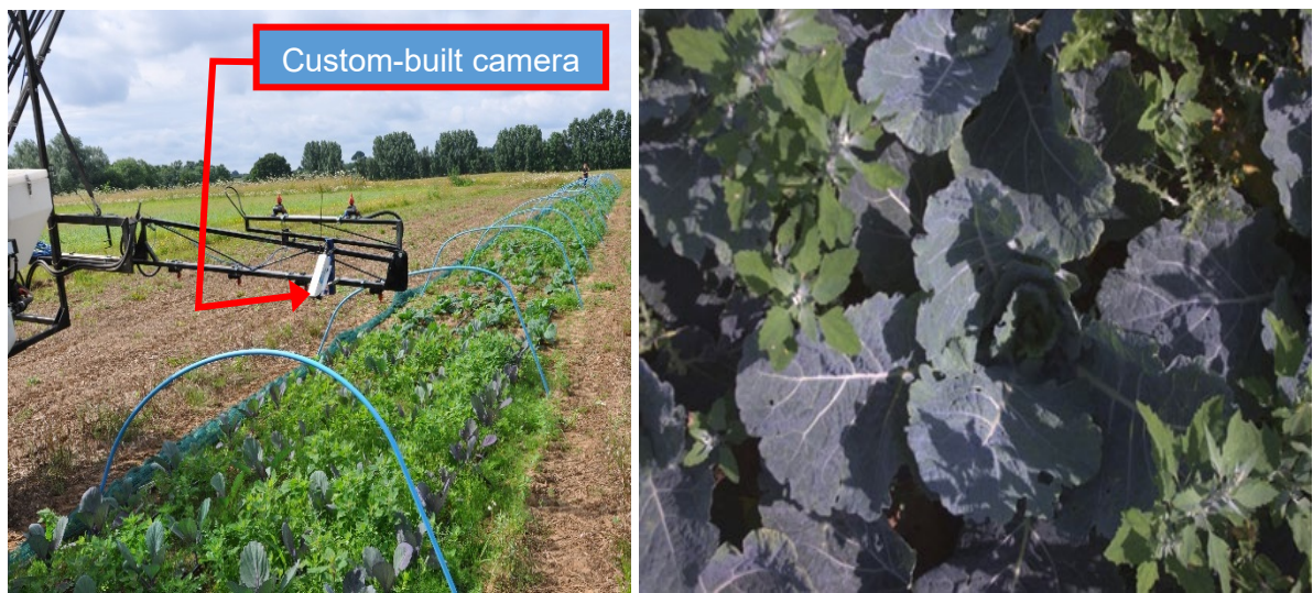
Figure 18 Custom-built camera system mounted on the boom of a small-plot sprayer, capturing images of weeds and red cabbage crop (left). Example of an image of a weedy plot with red cabbages as captured by the camera (right). The hoops were to support fleece.
